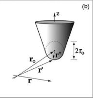
**Figure 7** (a) Induced surface-charge density on the surface of a laser-irradiated gold tip captured at a certain instance of time. Polarization along the tip axis gives rise to a large surface-charge accumulation at the tip's apex. The solid line indicates the tip geometry, whereas the shaded areas represent the surface charge. From Reference 27. (b) Coordinates used for the dipole model.
