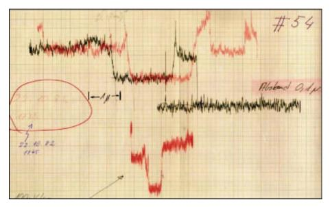
**Figure 3** Early near-field optical scan trace recorded with an aperture-type probe. The data are from the laboratory book of Winfried Denk, then working with Dieter W. Pohl at the IBM Research Laboratory in Switzerland. (Figure courtesy of Dieter W. Pohl)
