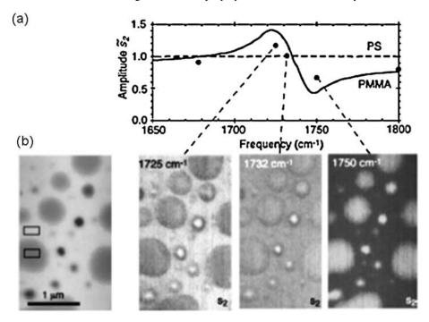
**Figure 12** Infrared scattering-type NSOM contrast of polystyrene (PS) inclusions in a polymethylmetacrylate (PMMA). (a) The calculated and measured contrast as a function of wavelength. (b) Images of the topography (*left*) and recorded infrared amplitudes (*right*). From Reference 90.
