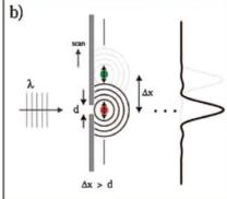
**Figure 2** Comparison of diffraction-limited optical microscopy and near-field optical microscopy. (a) Schematic representation of the diffraction limit showing the minimum detectable separation of two light scatterers. (b) Schematic of aperture scanning near-field microscopy. To first approximation, resolution is defined by the aperture size and not by the wavelength of the exciting radiation.
