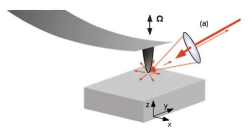
**Figure 9** Basic experimental setup of a scattering-type near-field scanning optical microscope. The tip of an atomic force–microscope cantilever operating in tapping mode is illuminated by a focused laser (*red arrow*). Scattering from the tip is collected by a lens and detected at the tapping-mode frequency ( $\Omega$ ). Modified from Reference 78.
