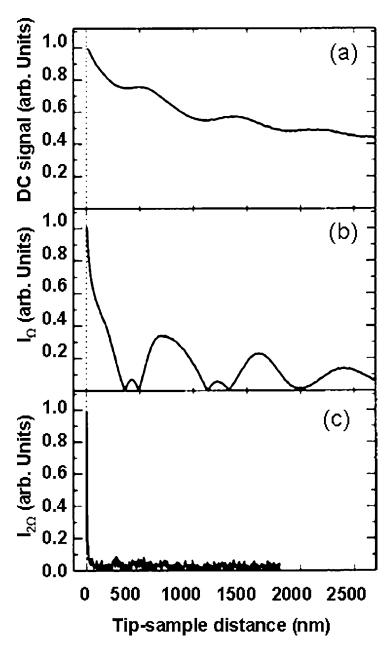
**Figure 10** The optical signal amplitudes, DC signal (*a*), at the tapping-mode frequency (*b*) and at the second harmonic (*c*). At the second harmonic, the detected optical signal is highly localized at the surface, and nonlocalized scattering is virtually eliminated. From Reference 85.
