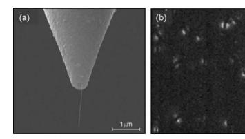
**Figure 13** (a) Scanning electron microscopy image of a tip-on-aperture probe consisting of a  $SiO_x$  whisker grown directly on an aperture probe. (b) Fluorescence patterns of single molecules recorded with a tip-on-aperture probe. The centers of all molecules appear dark because of fluorescence quenching. From Reference 50.
