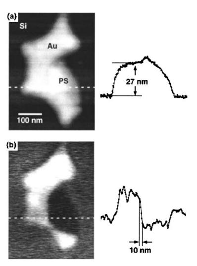
**Figure 11** Scattering-type NSOM images of the topography (*a*) and the simultaneously recorded optical amplitude (*b*) of a three-component test sample comprised of gold (Au) and polystyrene (PS) nanostructures on silicon (Si). The accompanying line scans of the regions detailed by the dashed lines in the image illustrate both the attainable resolution and the ability to distinguish between the nanometer-scale components, Au and PS, of this system. From Reference 89.
